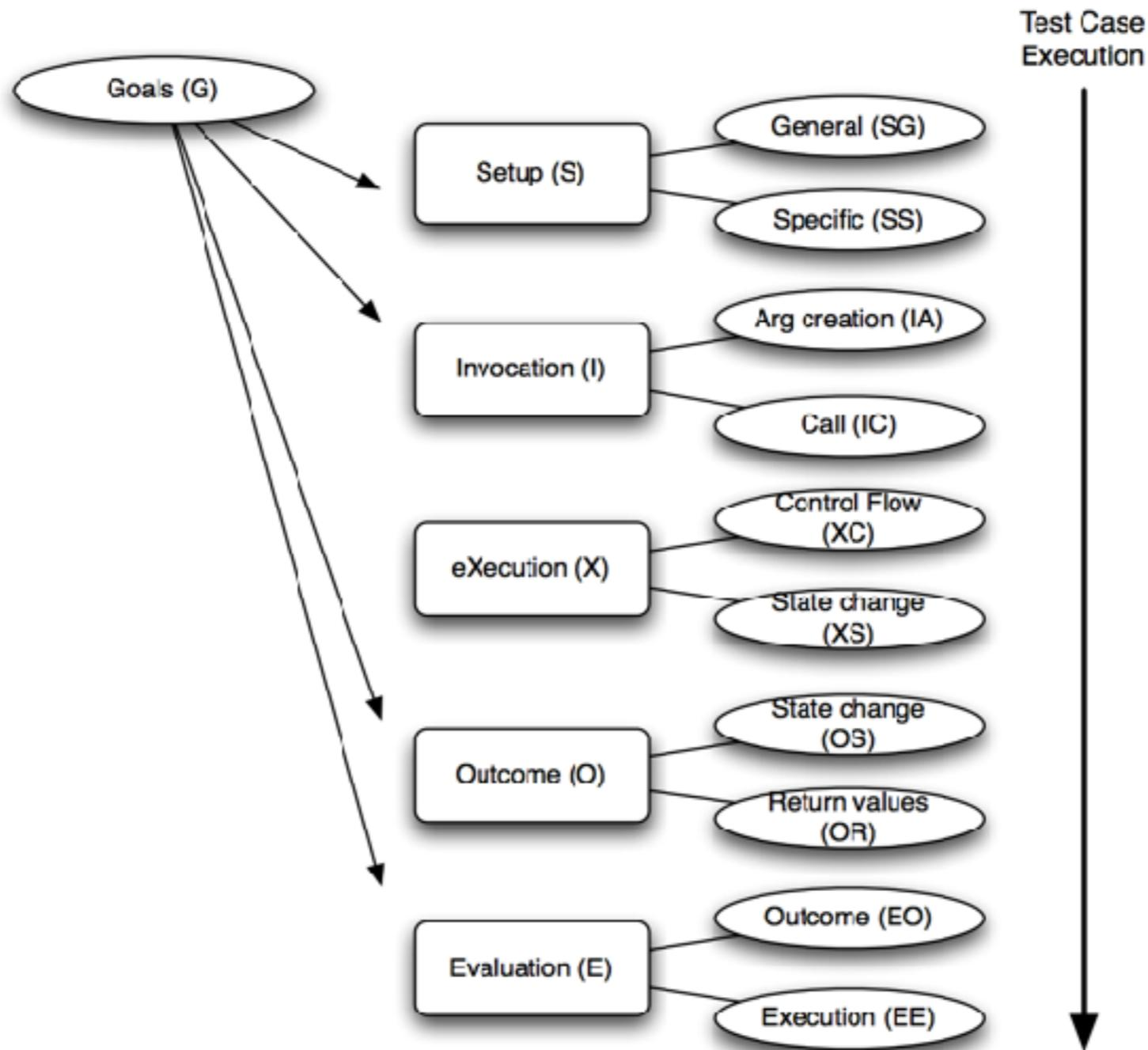
**VARIABILITY OF TESTS (VAT) Model of test information sources/types**
