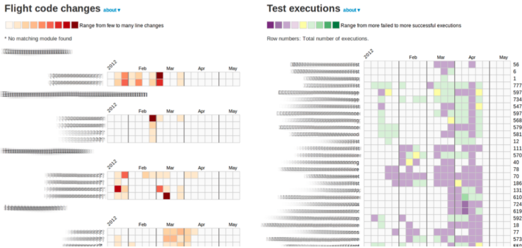
Fig. 4. Parts of prototype system dashboard with heatmaps integrating information about both source code changes and test outcomes.
